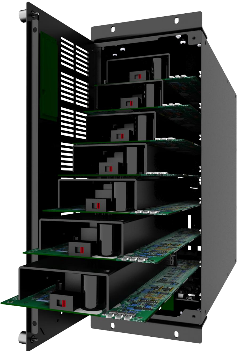
Illustration of Amp Cards Sliding into the Mainframe
